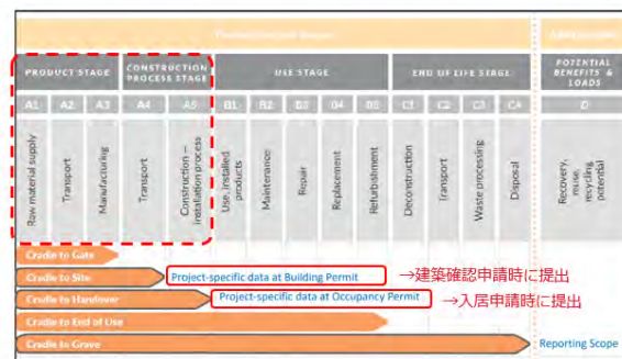
Figure 11 Recommended building system boundaries for embodied emissions assessments (Adapted from: Mistretta & Guerin, 2019) 図出典：Policy Research on Reducing the Embodied Emissions of New Buildings in Vancouver
